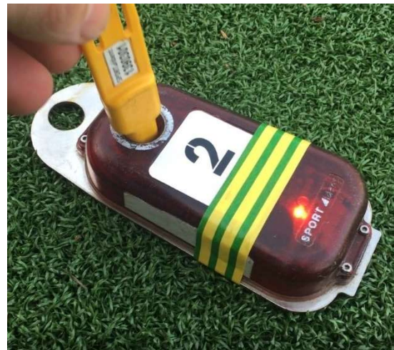
RED light flashes & control beeps when you dib your card (i.e. your visit is recorded)
