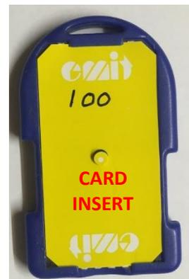
A small red LED light on the EMIT control will flash within less than a second of you correctly placing the card on the control (as shown in the adjacent picture). This tells you that your visit at this control has been registered and recorded on your EMIT card. Once you've seen the red LED light flash once, remove your card and move away from the control.
